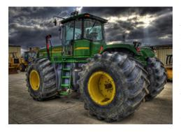
Modern day tractors maintain the classic look with the cab in the middle and engine in front, but have an enclosed cab and can have one of several different wheel styles.
