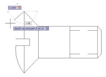
11 Move the cursor down to the location shown in the following figure. When the colored square appears and "endpoint" appears in the dynamic input cursor, click in the center of the square to complete the arc.
