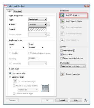
3 Click *inside* the polygon to select it. Do not select an edge of the polygon. Press the Enter key.
