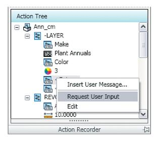
boxes except for the Layer Manager and Properties dialog boxes. All other commands with dialog boxes need to be run at the command line, with a dash [-] in front of the command. For example: -HATCH. The macro can get you into a dialog box, but you will need to enter any information and exit manually.
