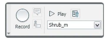
The Action Recorder records actions from the command line, toolbars, ribbon panels, pull-down menus, the Properties window, the Layer Properties Manager, and the Tool palette. After you are finished with your task, simply click the Stop button. You are prompted for a Macro Name, and a text version of your macro appears in a box for you to view. A file with an extension of *.actm* is then saved to the directory indicated in Options.
