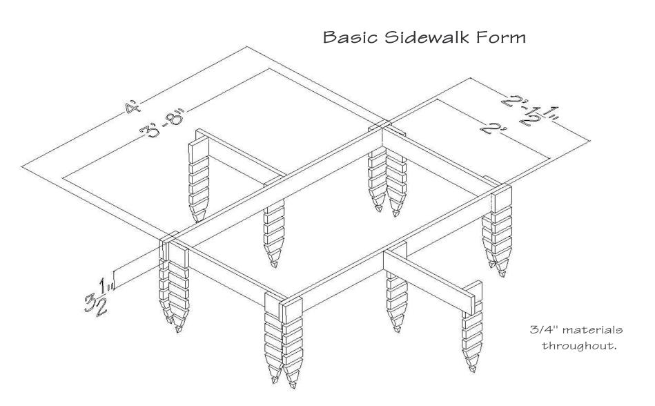
Start with an 18" stake. Drive into the ground until further movement is difficult. Level and adjust form. Attach stake to form. Cut top of stake flush with top of form.
