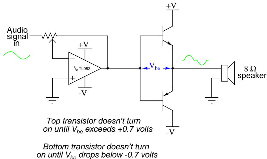
If you have already constructed the amplifier circuit in its final form, you may simplify it to this form and listen to the difference in sound quality. If you have not yet begun construction of the circuit, the schematic diagram shown above would be a good starting point. It will amplify an audio signal, but it will sound horrible!
