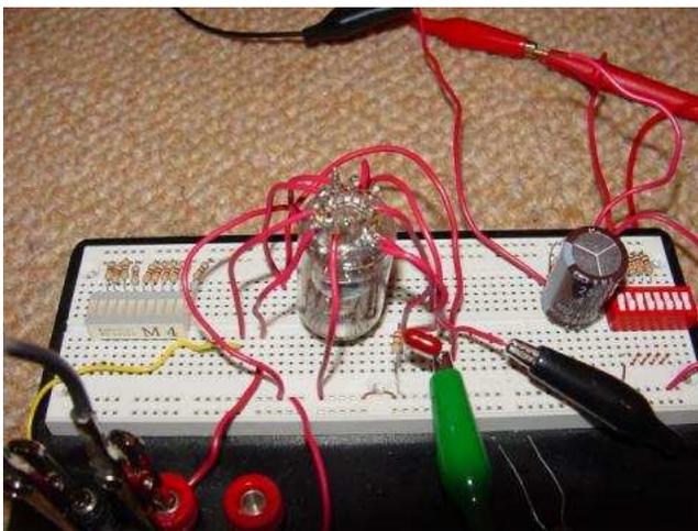
One benefit of mounting the tube in this position is ease of pin identification, since most "pin connection diagrams" for tubes are shown from a bottom view:
