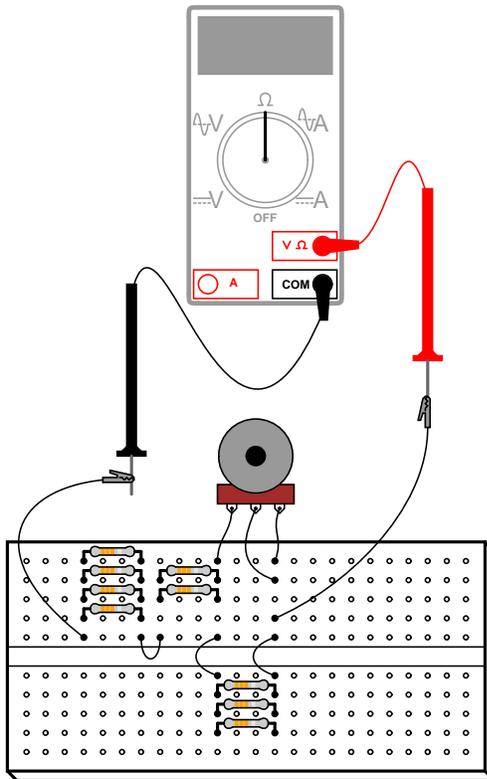
Creating a custom resistance range from fixed-value resistors and a potentiometer is a very useful technique for producing precise resistances required for certain circuits, especially meter circuits. In many electrical instruments – multimeters especially – resistance is the determining factor for the instrument's range of measurement. If an instrument's internal resistance values are not precise, neither will its indications be. Finding a fixed-value resistor
