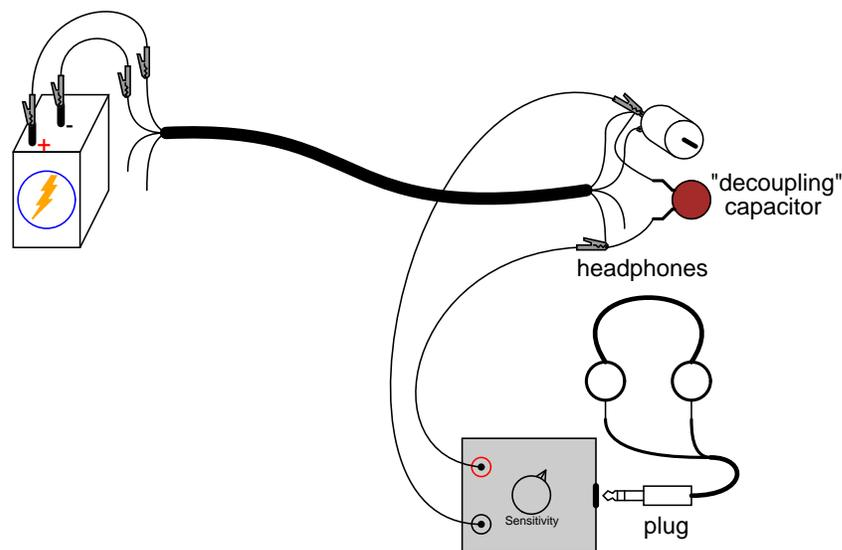
The *decoupling capacitor* acts as a practical short-circuit to any AC noise voltage, while not affecting DC voltage signals between those two points at all. So long as the decoupling capacitor value is significantly larger than the stray "coupling" capacitance between the cable's conductors, the AC noise voltage will be held to a minimum.
