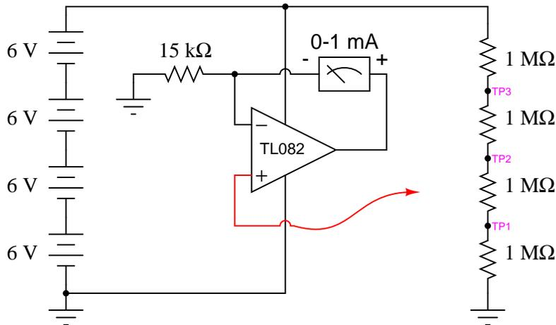
This alteration in the power supply increases the voltages at TP1, TP2, and TP3 to 6, 12, and 18 volts, respectively. With a 15 kΩ range resistor and a 1 mA meter movement, measuring 18 volts will gently "peg" the meter, but you should be able to measure the 6 and 12 volt test points just fine.
