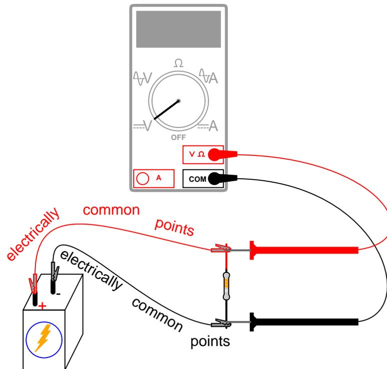
All points of contact along the upper wire in the illustration (colored red) are electrically common to each other. All points of contact along the lower wire (colored black) are likewise electrically common to each other. Voltage measured between any point on the upper wire and any point on the lower wire should be the same. Voltage measured *between any two common points*, however, should be zero.
