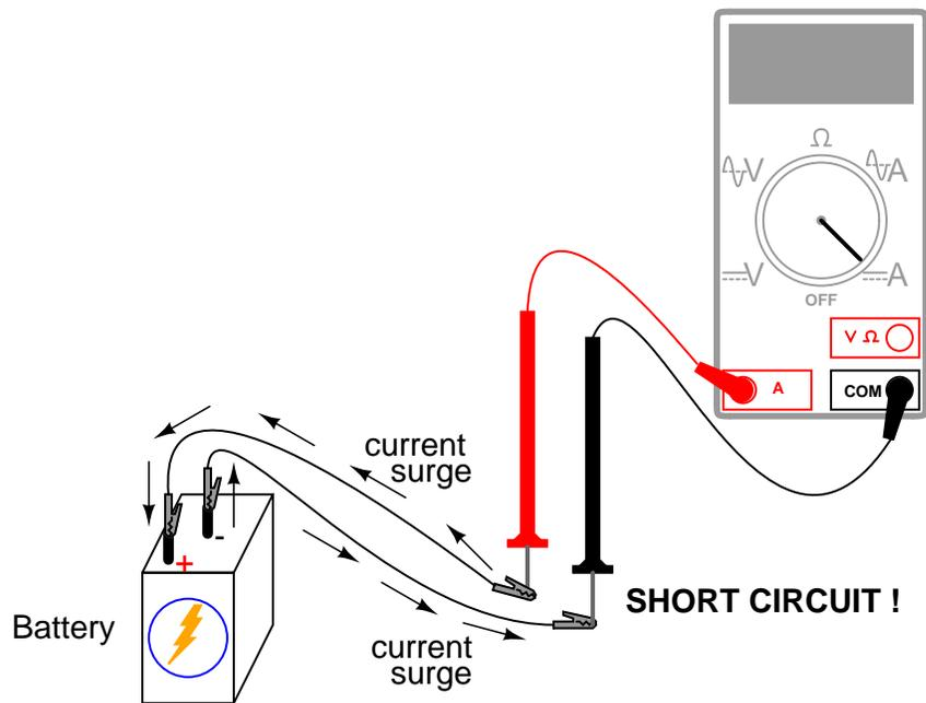
Ammeters are generally protected from excessive current by means of a small *fuse* located inside the meter housing. If the ammeter is accidentally connected across a substantial voltage source, the resultant surge in current will "blow" the fuse and render the meter incapable of measuring current until the fuse is replaced. **Be very careful to avoid this scenario!**
