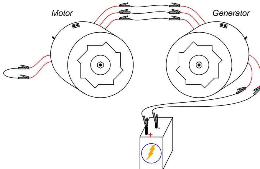
Spin the generator shaft while watching the motor shaft's rotation. Try reversing any *two* of the three-phase line connections between the two units and spin the generator again. What is different this time?
