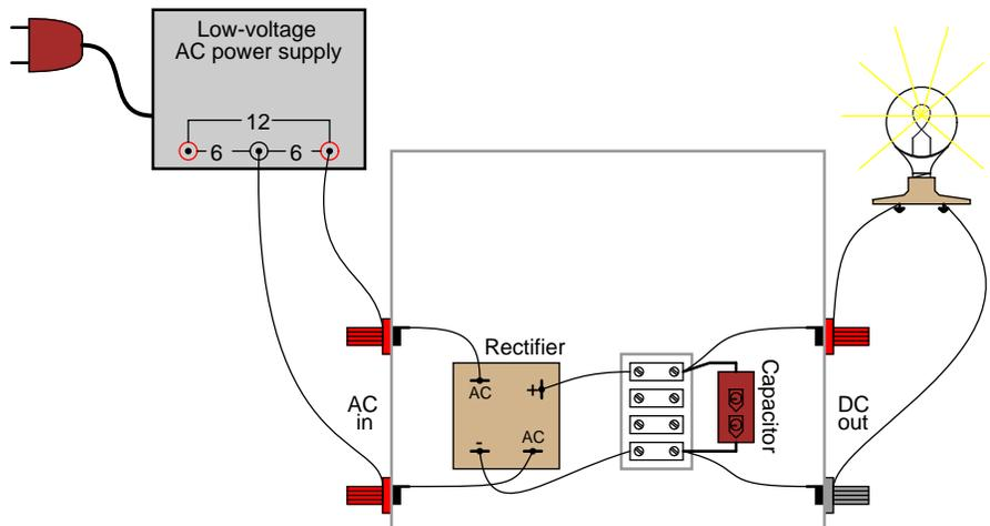
Re-measure the ripple voltage present between the rectifier/filter unit's "DC out" terminals. With a heavy load, the filter capacitor becomes discharged between rectified voltage peaks, resulting in greater ripple than before:
