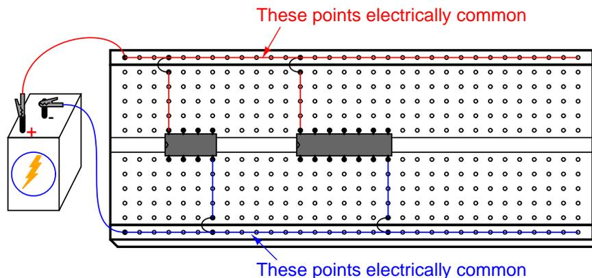
With so many of these integrated circuits having "reset," "enable," and "disable" terminals needing to be maintained in a "high" or "low" state, not to mention the  $V_{DD}$  (or  $V_{CC}$ ) and ground power terminals which require connection to the power supply, having both terminals of the power supply readily available for connection at any point along the board's length is very useful.
