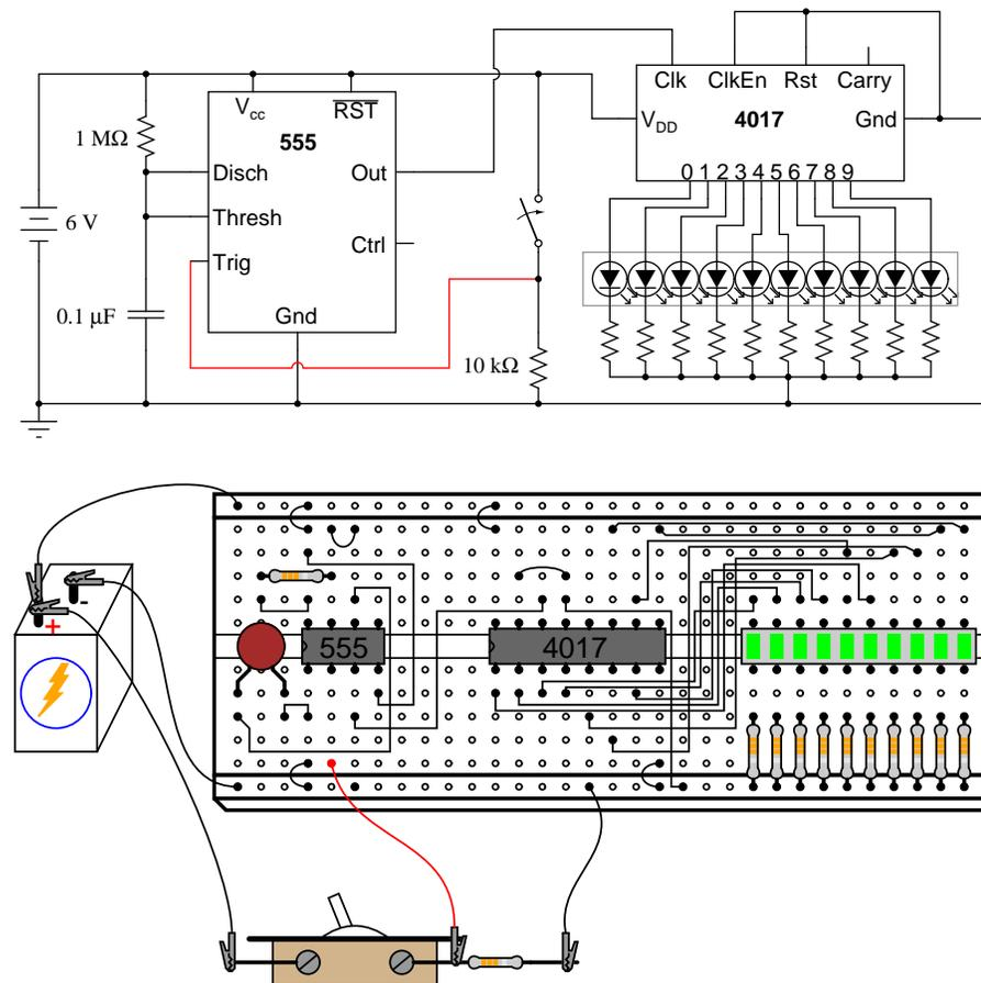
Please note that since we are using the 555 once again to provide a clock signal to the 4017, we must re-connect pin #3 of the 555 chip to pin #14 of the 4017 chip! Also, if you have altered the values of the resistor or capacitor in the 555 timer circuit, you should return to the original 1 MΩ and 0.1 μF components.
