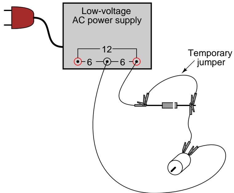
As you can see, permanent-magnet "DC" motors do not function well on alternating current. Remove the temporary jumper wire and reverse the diode's orientation in the circuit. Note the effect on the motor.
