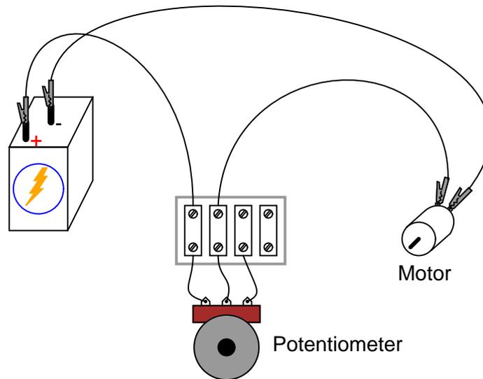
Moving the potentiometer control in the direction that brings the wiper closest to the other used terminal results in a lower resistance. The direction of motion required to increase or decrease resistance may be changed by using a different set of terminals:
