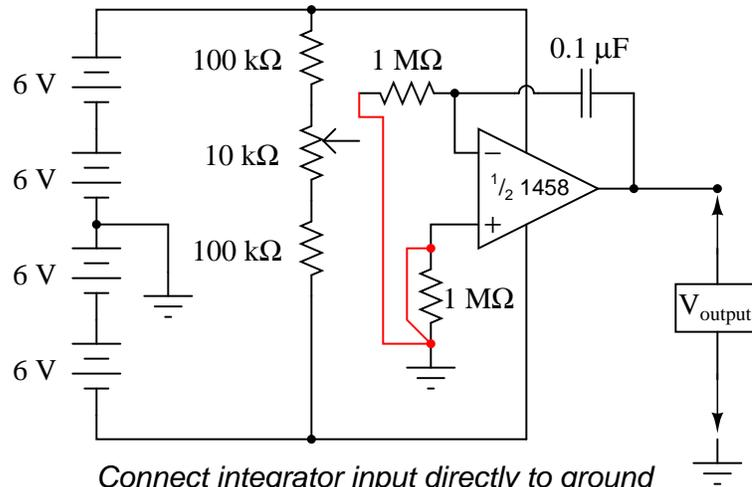
Connect integrator input directly to ground
