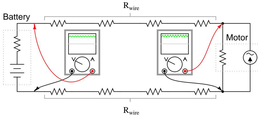
Use the audio detector to measure "noise" voltage directly across the battery. Since the AC noise is produced in this circuit by pulsating voltage drops along stray resistances, the less resistance we measure across, the less noise voltage we should detect:
