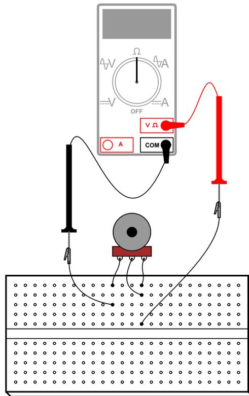
Suppose we wanted to elevate the lower end of this resistance range so that we had an adjustable range from  $10 \text{ k}\Omega$  to  $20 \text{ k}\Omega$  with a full sweep of the potentiometer's adjustment. This could be easily accomplished by adding a  $10 \text{ k}\Omega$  resistor in *series* with the potentiometer. Add one to the circuit as shown and re-measure total resistance while adjusting the potentiometer:
