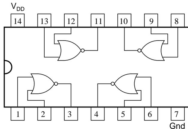
When two NOR gates are cross-connected as shown in the schematic diagram, there will be positive feedback from output to input. That is, the output signal tends to maintain the gate in its last output state. Just as in op-amp circuits, positive feedback creates *hysteresis*. This tendency for the circuit to remain in its last output state gives it a sort of "memory." In fact, there are solid-state computer memory technologies based on circuitry like this!
