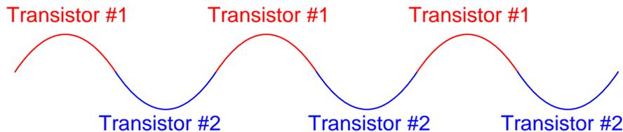
If the "hand-off" between the two transistors is not precisely synchronized, though, the amplifier's output waveform may look something like this instead of a pure sine wave:
