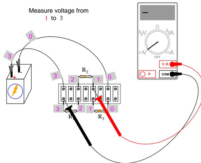
Try stepping between any set of points, in any order, around your circuit and see for yourself that the algebraic sum always equals zero. This Law holds true no matter what the configuration of the circuit: series, parallel, series-parallel, or even an irreducible network.
