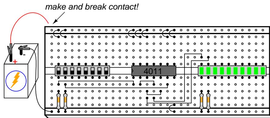
When a latch circuit such as this is powered up into its "latched" state, the gates race against each other for control. Given the "low" inputs, both gates try to output "high" signals. If one of the gates reaches its "high" output state before the other, that "high" state will be fed back to the other gate's input to force its output "low," and the race is won by the faster gate.
