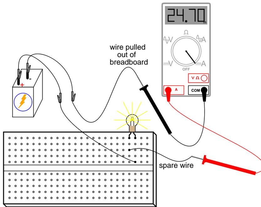
Again, measure current through different wires in this circuit, following the same connection procedure outlined above. What do you notice about these current measurements? The results in the breadboard circuit should be the same as the results in the free-form (no breadboard) circuit.
