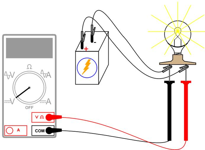
The voltmeter should register a voltage lower than the usual voltage of the battery. If you use your voltmeter to read the voltage directly at the battery terminals, you will measure a low voltage there as well. Why is this? The large current drawn by the high-power lamp causes the voltage at the battery terminals to "sag" or "droop," due to voltage dropped across resistance internal to the battery.
