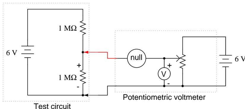
The circle symbol with the word "null" written inside represents the null detector. This can be any arbitrarily sensitive meter movement or voltage indicator. Its sole purpose in this circuit is to indicate when there is *zero* voltage: when the adjustable voltage source (potentiometer) is precisely equal to the voltage drop in the circuit under test. The more sensitive this null detector is, the more precisely the adjustable source may be adjusted to equal the voltage
