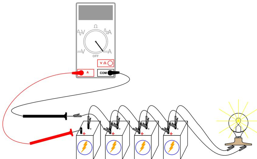
By breaking the circuit for just one battery, and inserting our ammeter within that break, we intercept the current of that one battery and are therefore able to measure it. Measuring total current involves a similar procedure: make a break somewhere in the path that total current must take, then insert the ammeter within than break:
