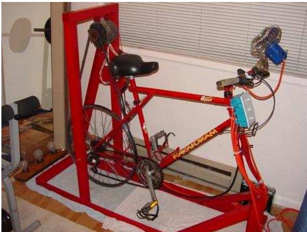
You can see a bank of three 12-volt "RV" light bulbs behind the bicycle unit (in the lower-left corner of the photograph), which I use for a load when riding the bicycle as an exercise machine. A set of three switches is mounted at the front of the bicycle, where I can turn loads
