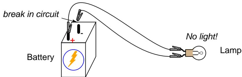
Using your multimeter set to the appropriate "DC volt" range, measure voltage across the battery, across the lamp, and across each jumper wire. Familiarize yourself with the normal voltages in a functioning circuit.
