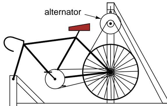
The rear wheel drives the generator sheave with a *long v-belt*. This belt also supports the rear of the bicycle, maintaining a constant tension when a rider is pedaling the bicycle. The generator hangs from a steel support structure (I used welded 2-inch square tubing, but a frame could be made out of lumber). Not only is this machine practical, but it is reliable enough to be used as an exercise machine, and it is inexpensive to make:
