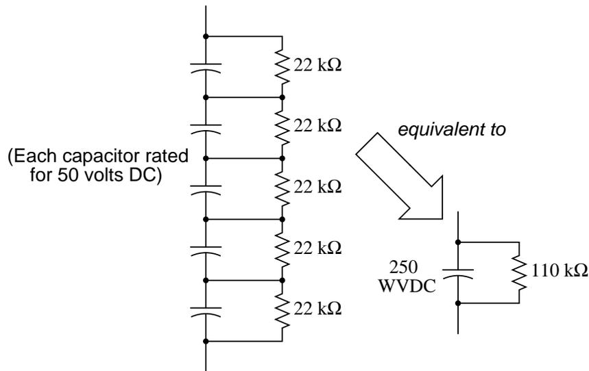
Bear in mind that the total capacitance for this five-capacitor network will be  $1/5$ , or 20%, of each capacitor's value. Also, to ensure even charging of capacitors in the network, be sure all capacitor values (in  $\mu\text{F}$ ) and all resistor values are identical.
