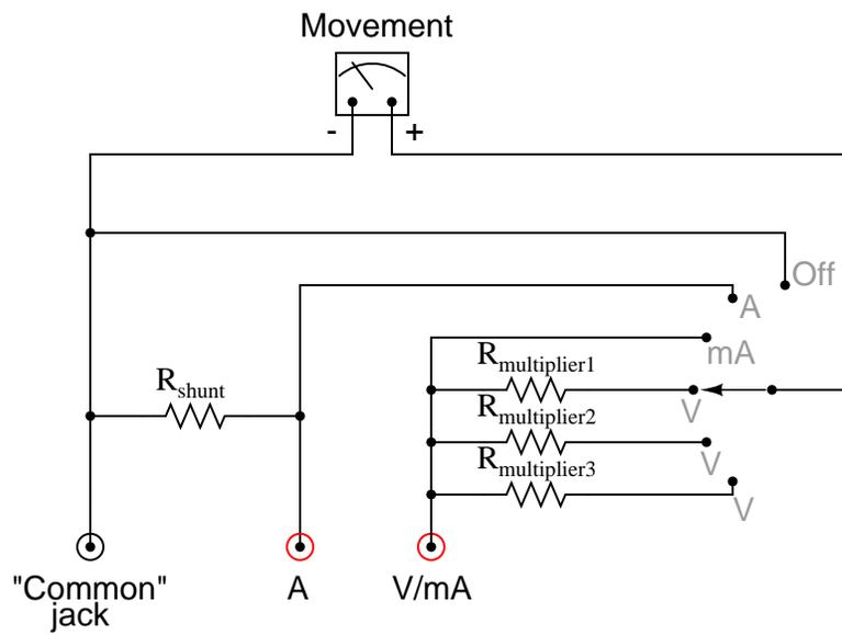
" $R_{multiplier}$ " resistors are actually rheostat networks
