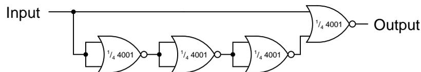
Normally, when using a NOR gate as an inverter, one input would be grounded while the other acts as the inverter input, to minimize input capacitance and increase speed. Here, however, slow response is *desired*, and so I parallel the NOR inputs to make inverters rather than use the more conventional method.
