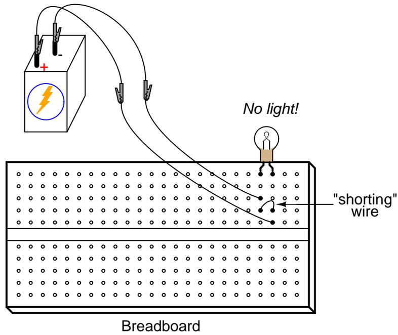
Here is an example of an *accidental* short circuit of the type typically made by students unfamiliar with breadboard usage:
