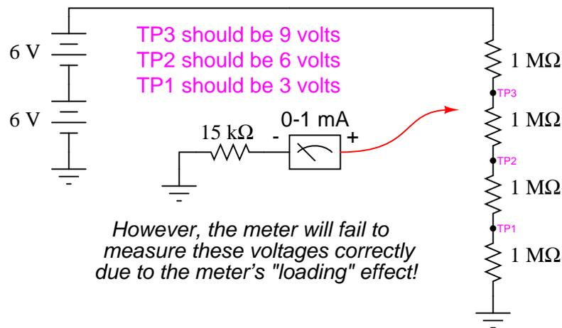
Try using the meter movement and  $15\text{ k}\Omega$  resistor as shown to measure these three voltages. Does the meter read falsely high or falsely low? Why do you think this is?
