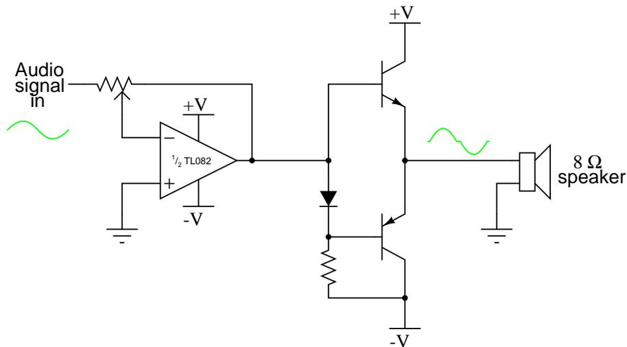
Since the voltage drop of a single diode will always be less than the combined voltage drops of the two transistors' base-emitter junctions, the transistors can never turn on simultaneously, thereby preventing class AB operation. Next, to help get rid of the remaining crossover distortion, the feedback signal of the op-amp is taken from the output terminal of the amplifier (the transistors' emitter terminals) like this:
