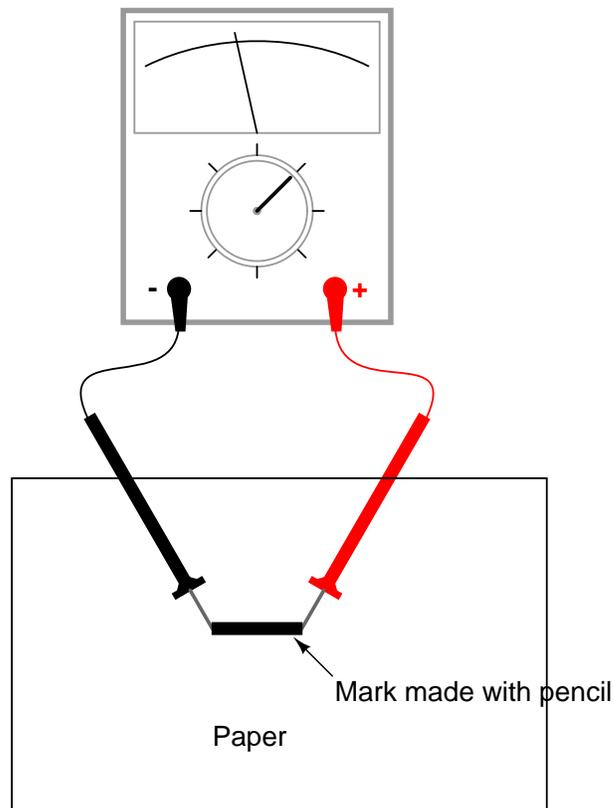
Move the probe tips closer together on the black mark and note the change in resistance value. Does it increase or decrease with decreased probe spacing? If the results are inconsistent, you need to redraw the mark with more and heavier pencil strokes, so that it is consistent
