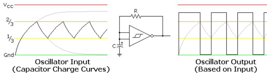
**555 Oscillator Waveforms**
