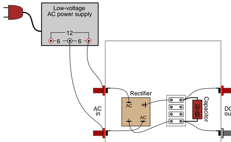
Measure the AC voltage output by the low-voltage power supply. Your meter should indicate approximately 6 volts if the circuit is connected as shown. This voltage measurement is the RMS voltage of the AC power supply.
