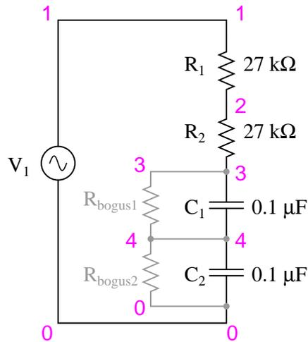
The two large-value resistors  $R_{bogus1}$  and  $R_{bogus1}$  are connected across the capacitors to provide a DC path to ground in order that SPICE will work. This is a "fix" for one of SPICE's quirks, to avoid it from seeing the capacitors as open circuits in its analysis. These two resistors are entirely unnecessary in the real circuit.
