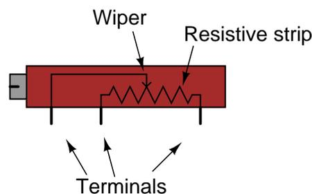
It should be noted that not all linear potentiometers have the same pin assignments. On some, the middle pin is the wiper.
