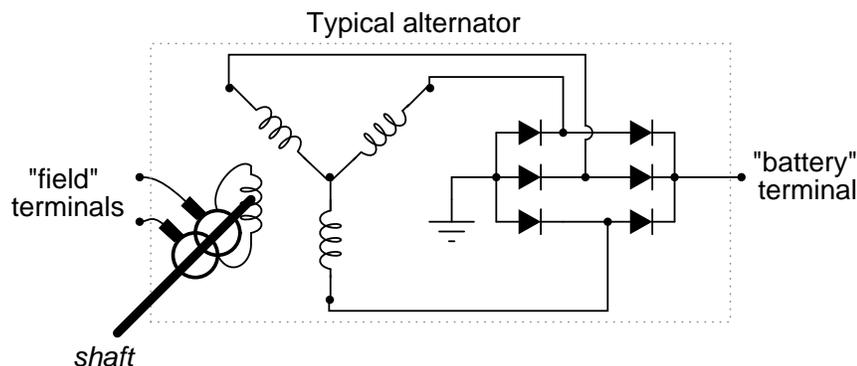
An automotive alternator is a three-phase generator with a built-in rectifier circuit consisting of six diodes. As the sheave (most people call it a "pulley") is rotated by a belt connected
