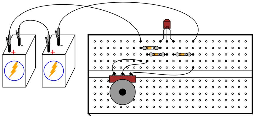
Repeat the same voltage measurement and recording exercise with the 1.5 kΩ resistor installed, calculating the new (reduced) voltage gain. Try altering the transistor's temperature again and noting the output voltage for a steady input voltage. Does it change more or less than without the 1.5 kΩ resistor?
