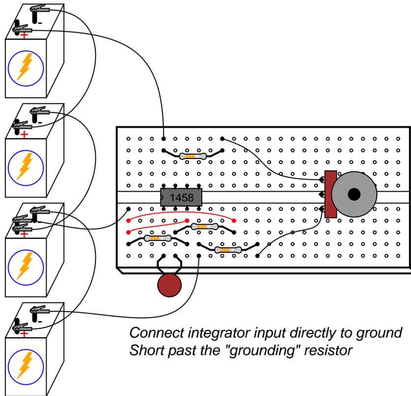
Connect integrator input directly to ground
