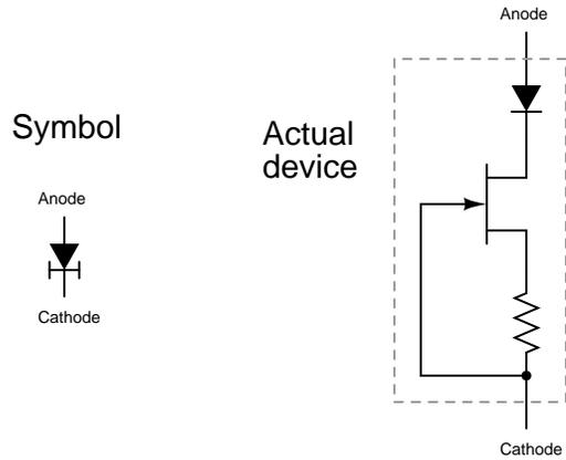
A normal PN-junction diode is included in series with the JFET to protect the transistor against damage from reverse-bias voltage, but otherwise the current-regulating facility of this device is entirely provided by the field-effect transistor.
