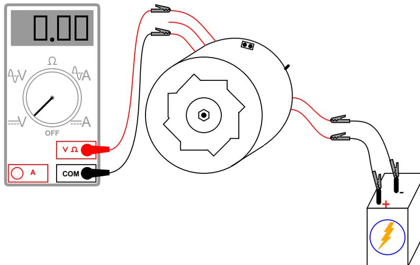
With the multimeter set to the "DC volts" function, *slowly* rotate the alternator shaft. The voltmeter reading should alternate between positive and negative as the shaft is turned: a demonstration of very slow alternating voltage (AC voltage) being generated. If this test is successful, switch the multimeter to the "AC volts" setting and try again. Try spinning the shaft slow and fast, comparing voltmeter readings between the two conditions.
