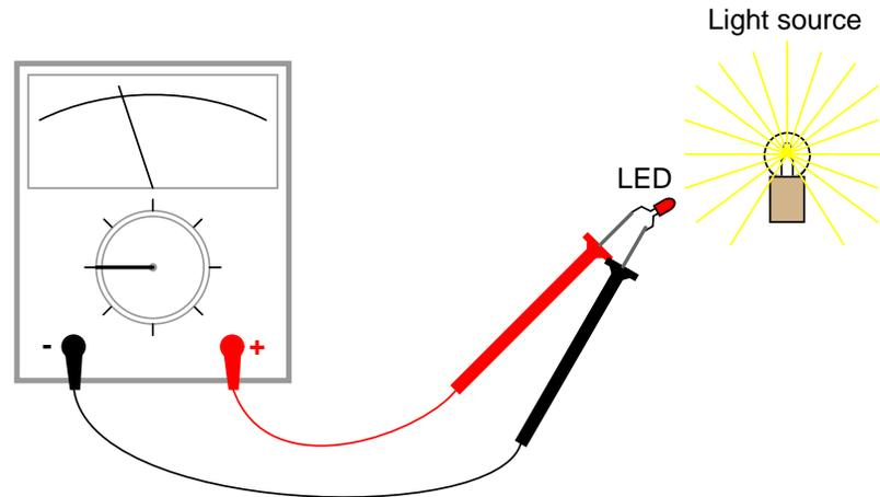
Batteries develop electrical voltage through chemical reactions. When a battery "dies," it has exhausted its original store of chemical "fuel." The LED, however, does not rely on an internal "fuel" to generate voltage; rather, it *converts* optical energy into electrical energy. So long as there is light to illuminate the LED, it will produce voltage.
