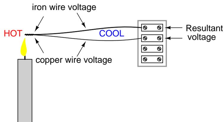
Thermocouples are widely used as temperature-sensing devices because the mathematical relationship between temperature difference and resultant voltage is both repeatable and fairly linear. By measuring voltage, it is possible to infer temperature. Different ranges of temperature measurement are possible by selecting different metal pairs to be joined together.
