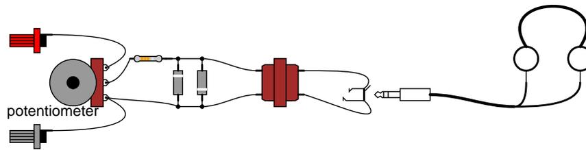
Adjust the 100 k $\Omega$  voltage divider potentiometer to about mid-range when initially sensing a voltage signal of unknown magnitude. If the sound is too loud, turn the potentiometer down and try again. If too soft, turn it up and try again. The detector produces a "click" sound whenever the test leads make or break contact with the voltage source under test. With my cheap headphones, I've been able to detect currents of less than 1/10 of a microamp ( $\approx 0.1 \mu\text{A}$ ).
