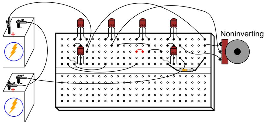
Note the triangular symbol of the op-amp shown in the lower schematic diagram. The inverting and noninverting inputs are designated with (-) and (+) symbols, respectively, with the output terminal at the right apex. The feedback wire connecting output to inverting input is shown in red in the above diagrams.
