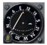
Notice that it doesn't matter which number we put at the top of the OBS. We could put the desired course, or its reciprocal, and the indications will not change. There is no reverse sensing.
