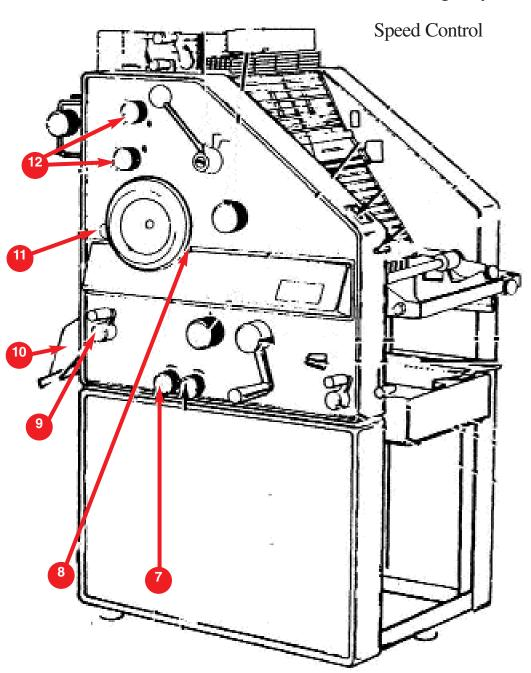
Aquamatic Control Aquamatic Night Latch Aquamatic Lock Out Latch Ink Fountain Control Knobs Ink Control Lever Operation Control Handel
